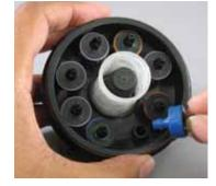
Helpful Hint: Always install emitters with the pointed end (inlet barb) or threaded end up, as shown
