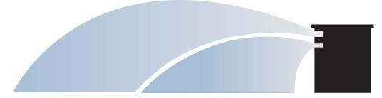
U-Series nozzles offer better, more uniform water distribution. Water flowing from both orifices combines to form a continuous water stream. Eliminates gaps for more uniform coverage throughout the entire watering area
