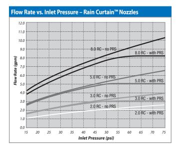
How much water can you save each minute using Rain Bird<sup>®</sup> 5000 PRS Rotors with Flow Optimizer Technology?
