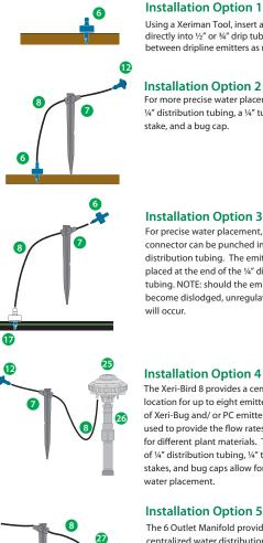
Using a Xeriman Tool, insert an emitter directly into 1/2" or 3/4" drip tubing or between dripline emitters as needed.
