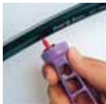
One Step Xeri-Bug™ Insertion
