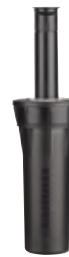
PROS-03 Overall height: 5" Pop-up height: 3" Exposed diameter: 2¼" Inlet size: ½" Female NPT
