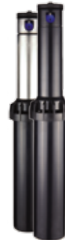
I-20-06 Overall height: 9¾" Pop-up height: 6" Exposed diameter: 1¾" Inlet size: ¾" female NPT
