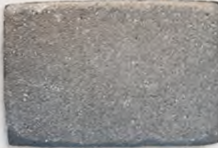
BELGARD COLORGARD PAVER AFTER 15 YEARS OF EXPOSURE
