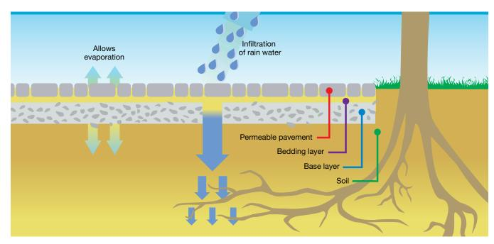
Illustration of the Unilock Permeable Pavement System.
